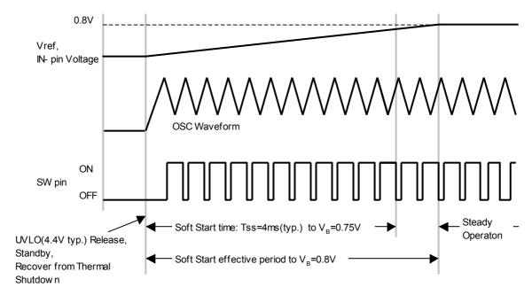
Fig. 1. Startup Timing Chart
